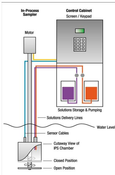
**Figure 3: Diagram of the In-situ Nutrient Analyzer**
