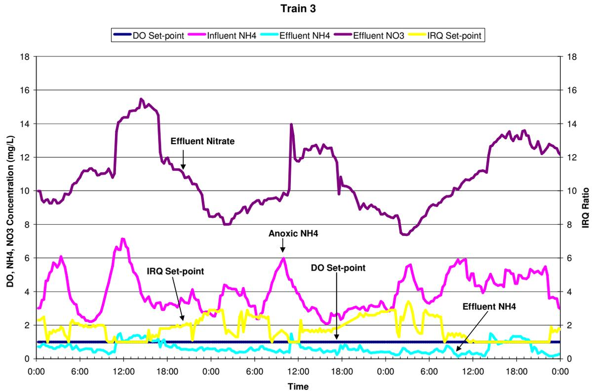
**Figure 8: Train 3 Typical DO and IRQ Set-point Control, Upgraded Process**
