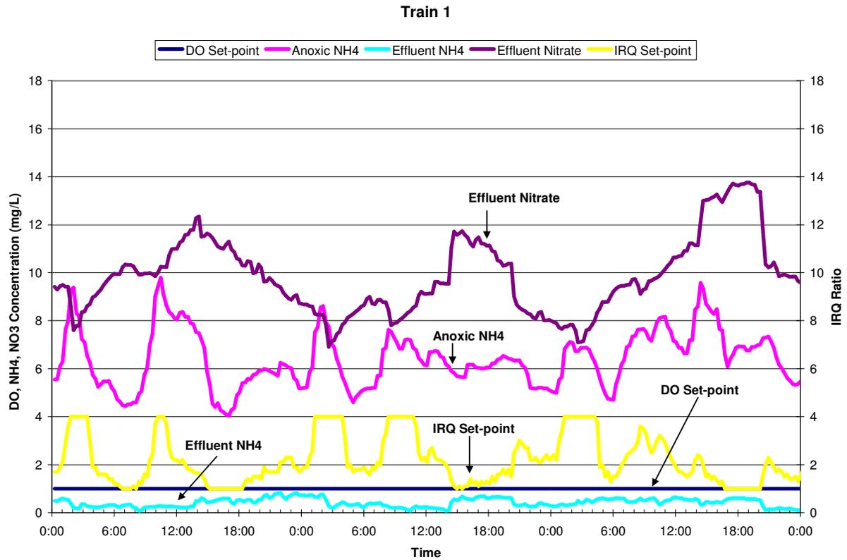
**Figure 7: Train 1 Typical DO and IRQ Set-point Control, Upgraded Process**
