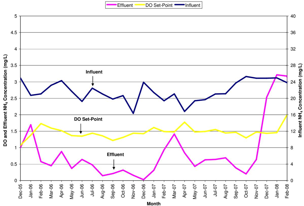
Figure 6: Monthly Average Influent Ammonia, Effluent Ammonia, and DO Set-point
