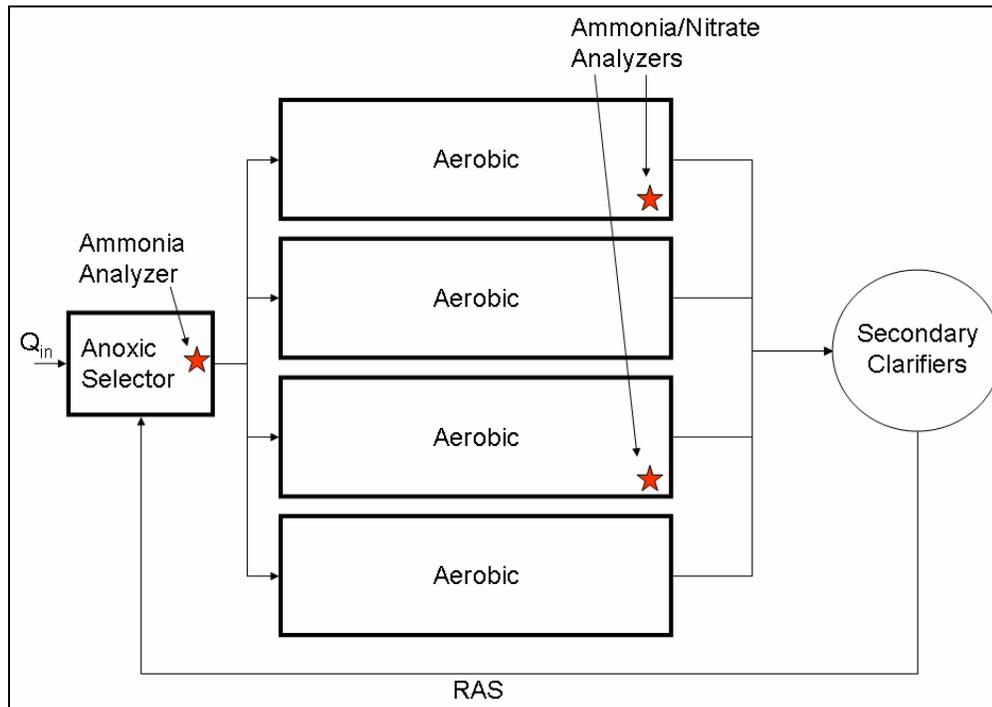
Figure 1: Original Process Layout
