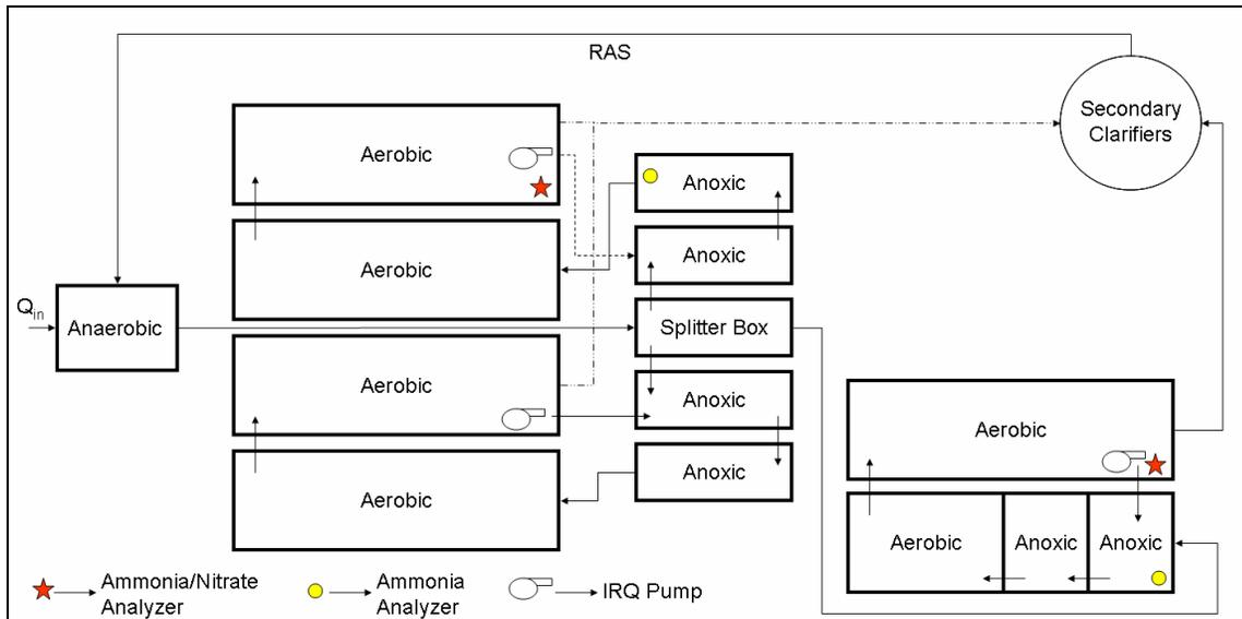
**Figure 2: Upgraded Process Layout** (IRQ = Internal Recycle Flow)
